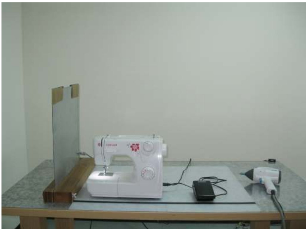
Picture 4: Test setup for Electrostatic Discharge
