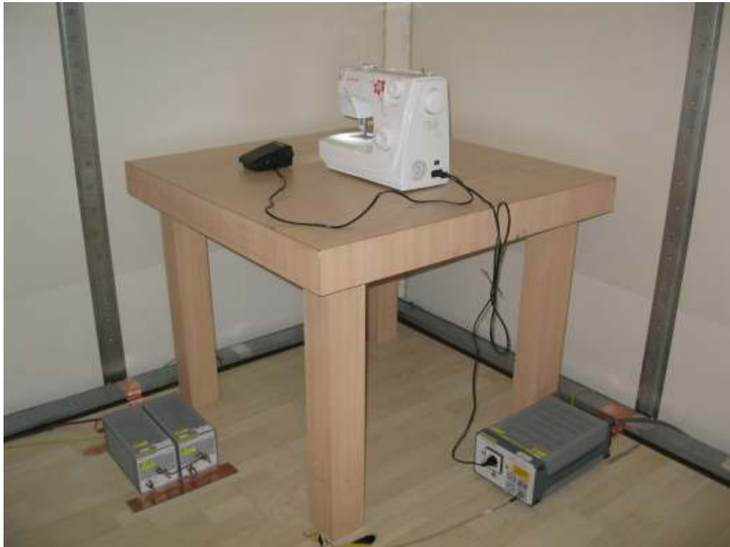
Picture 1: Test setup for Conducted Emission
