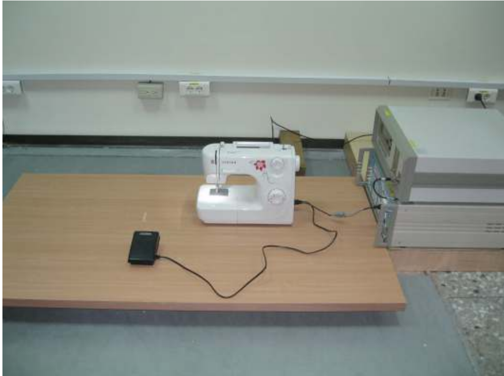
Picture 5: Test setup for Electrical Fast Transient
