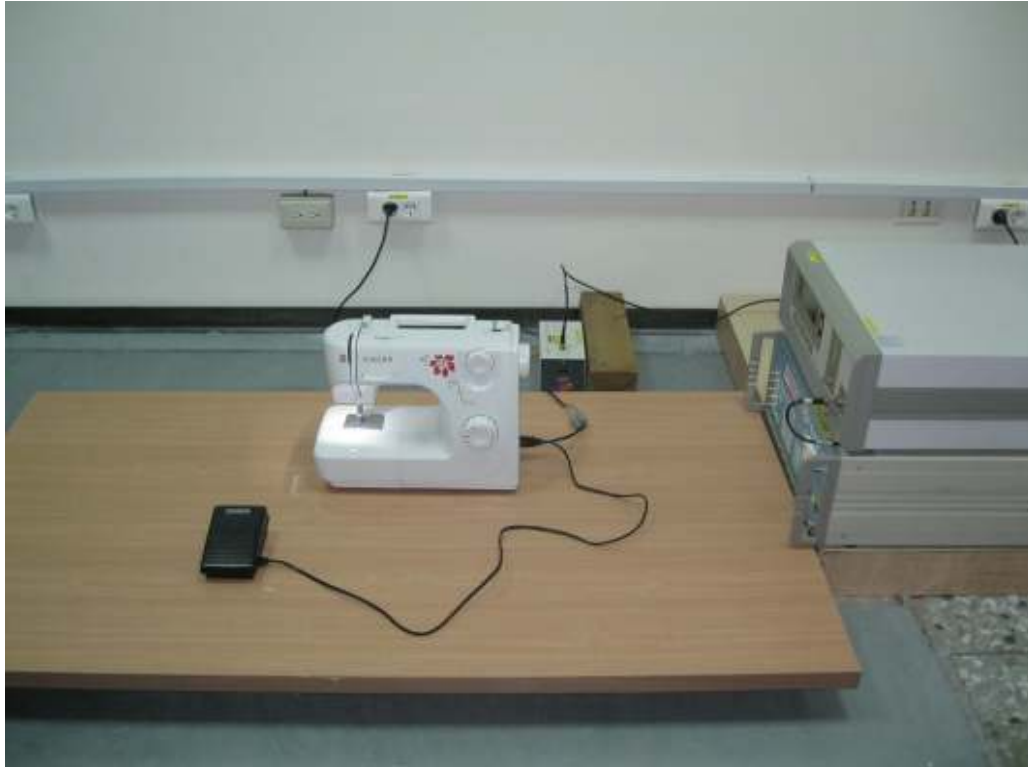
Picture 7: Test setup for Conducted Susceptibility
