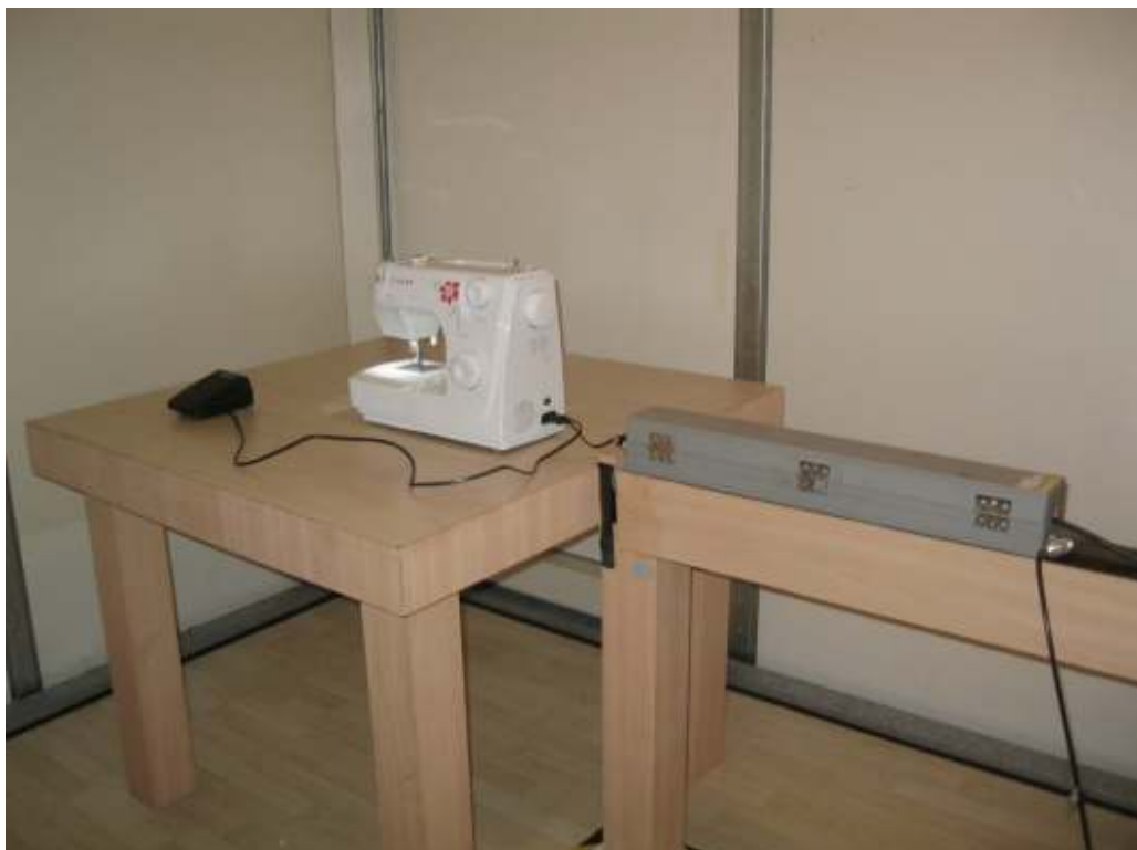
Picture 2: Test setup for Disturbance Power
