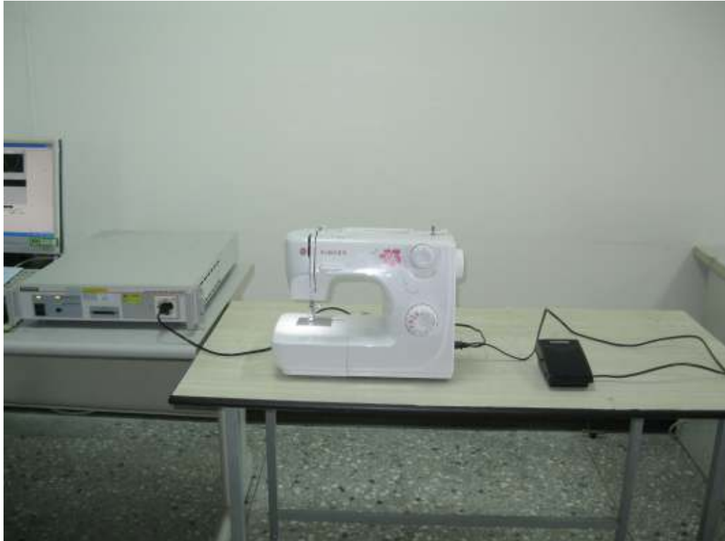
Picture 3: Test setup for Harmonics and Flicker
