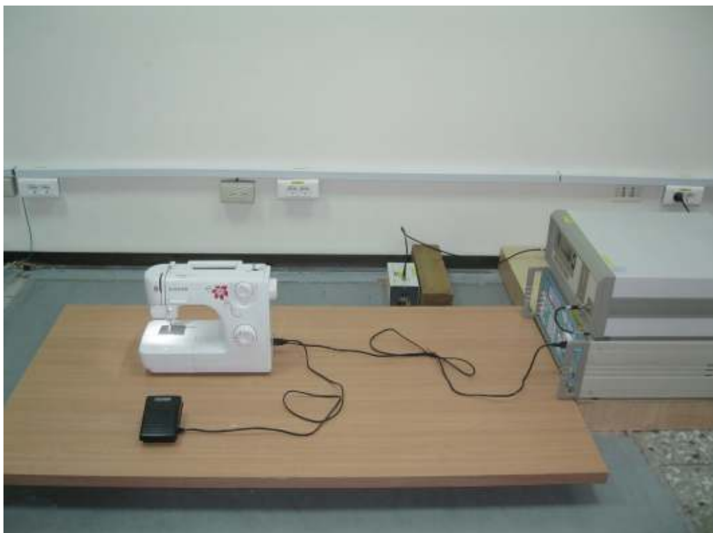
Picture 8: Test setup for Voltage Dips and Interruptions
