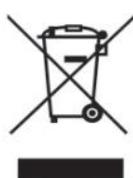
This product carries the recycling symbol for waste electrical and electronic equipment (WEEE). This means that this product must be processed in accordance with the European Directive 2012/19/EU so that it can be recycled or removed to limit its impact on the environment.
