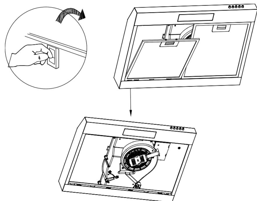
2. Insert the activated carbon insert into the position indicated in the figure.
