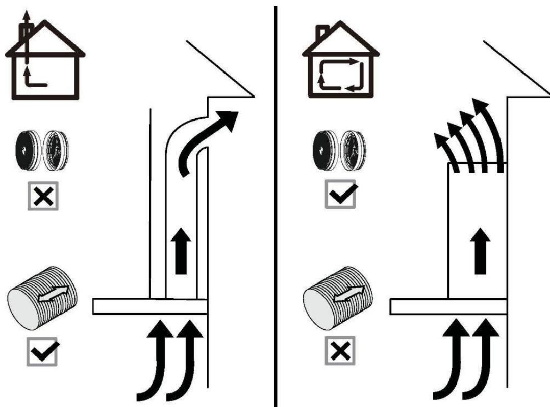
b) When possible, use at least 60cm straight runs before any turns. Larger duct work may be required for best performance with longer duct runs.
