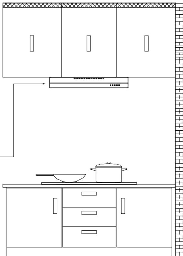
4) Align the air ventilation port of the cook hood with the cabinet ventilation hole at the bottom, pass the power cord through the power hole, and then use four 4 \* 20mm screws to lock into the corresponding position to fix the cook hood.
