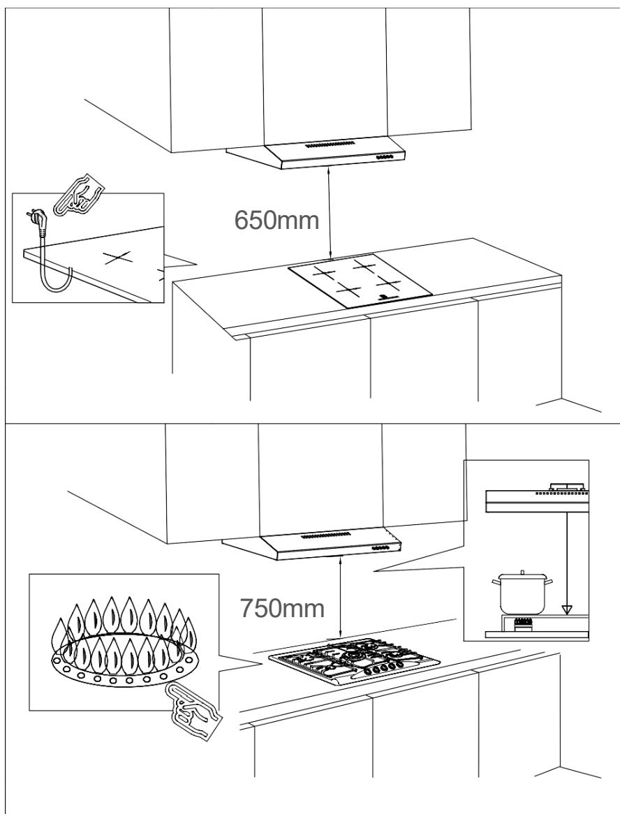
3) Put the outlet onto the cooker hood. Remove the aluminum grease filter, then put the cooker hood under the cabinet.
