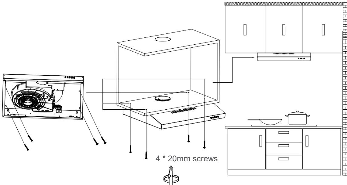
5) Install the air baffle and put the grease filter back on the cooker hood.
