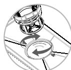
**C** You can put the filter back after cleaned. The cylinder filter should be assemble with clockwise until the triangle mark of filter, filter net and stainless steel in the same time.
