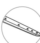
**B** Check if the spray arms blocked. If it does, please use a thin wire to pull the blockages out or flush the hole with water.
