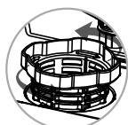
**A** Turn the cylinder filter out with anticlockwise.
