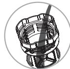
**B** Flush cylinder filter and filter net.
