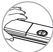
1. Press convex button on the detergent powder/tablet feeder
