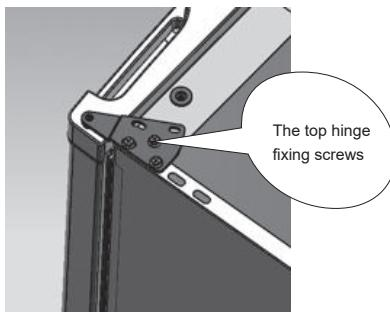
3. Place the top hinge, bushing and door stop on the other side.
