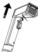
Press and hold the release button and pull outwards to remove the brush head
