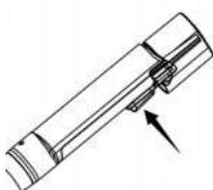
2. Press and hold the water control button to start self-cleaning
