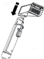
Insert the brush head in alignment and hear "click" sound, the installation is complete.
