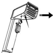
Hold the release button and pull outwards to remove the brush head module.
