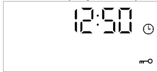
Pic 8: Door lock activated display effect under standby status
