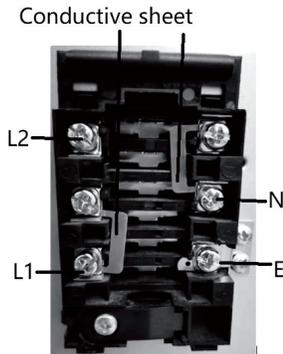
3, 380-415V 3N~: power cord requirements: wire diameter 5G 2.5mm<sup>2</sup> at least; cord type: H05RR-F, H05RN-F, H07RN-F. The conductive sheet connection method as below:
