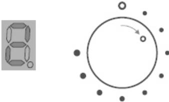
If you turn the knob to the "OFF" position, the power setting returns to "0". The maximum power of cooking zones is as follows:
