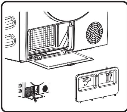
2. Turn the locking knob of the cover to unlock position.
