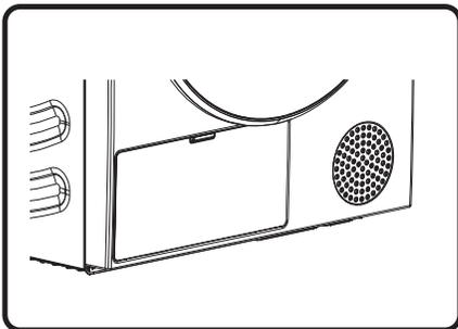
3. Install the inner door cover to the original positions, lock the knob and close the heat exchanger door cover.
