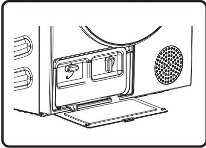
1. Pull the buckle of the heat exchanger door cover at the lower left to open the door cover.
