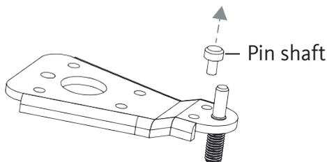
8. Insert the pin shaft into the left hole on the lower hinge.
