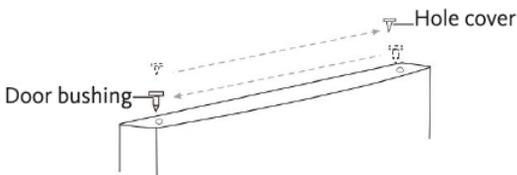
13. Remove the center hinge screw hole plugs on the left side of the cabinet, then install the plugs in the screw holes on the right side of the cabinet.
