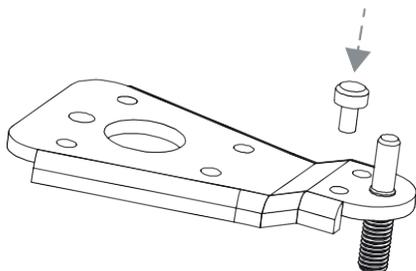
9. Install the lower hinge on the left side of the cabinet.
