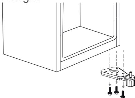
7. Remove the pin shaft from the right hole on the lower hinge.
