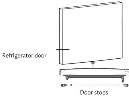
11. Install the refrigerator compartment door.
