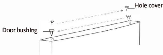
18. Remove the screw that secures the hinge screw hole cover from the top left side of the cabinet, remove the cover and secure the cover on the top right side of the cabinet
