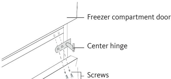
5. Remove the refrigerator compartment door.
