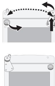
3. Put the door on bottom hinge, assemble the shaft of the top hinge as the follow picture and assemble the upper hinge, upper hinge cover and plastic screw hole caps successively.
