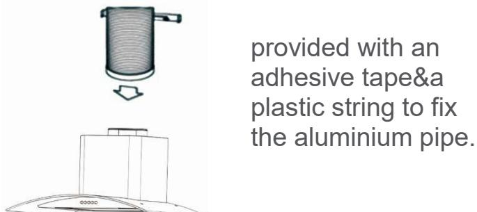
provided with an adhesive tape&a plastic string to fix the aluminium pipe.
