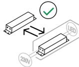
EN Replaceable control gear by an end-user
