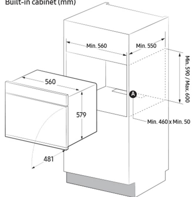
The built-in cabinet must have vents (A) to ventilate heat and circulate the air.
